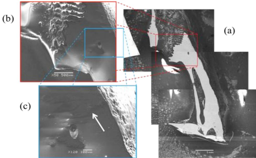
SEM images of the polished side-up section of plate Ba1c. (a) Compiled backscatter image of entire plate with holes and channels illustrated by dark regions; (b) higher magnification of an area of the plate with the secondary detector; (c) even greater magnification, showing visible dendritic structural lines toward the top (shown by arrow).
