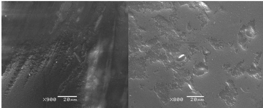
High magnification SEM secondary images of fine-grained dendritic structure on top-up sections of Ba1d (left) and Ba2 (right).
