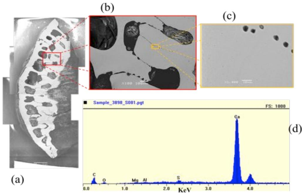
(a) Full SEM and EDS bottom-up section data on Ba1a; (b) increased magnification revealing 'zipper' structure; (c) even greater magnification image used for mapping EDS data; and (d) Ba1a EDS elemental data (with scale in keV).
