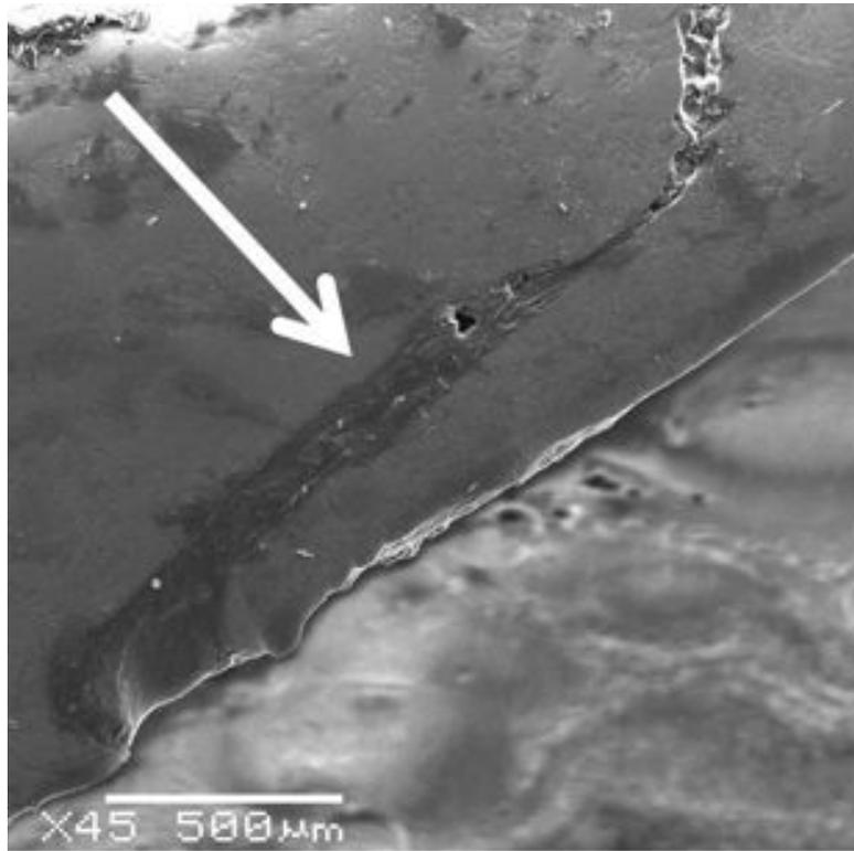
The layered connection between two exoskeleton plates on sample *Balanus amphitrite* 2 (Ba2).
